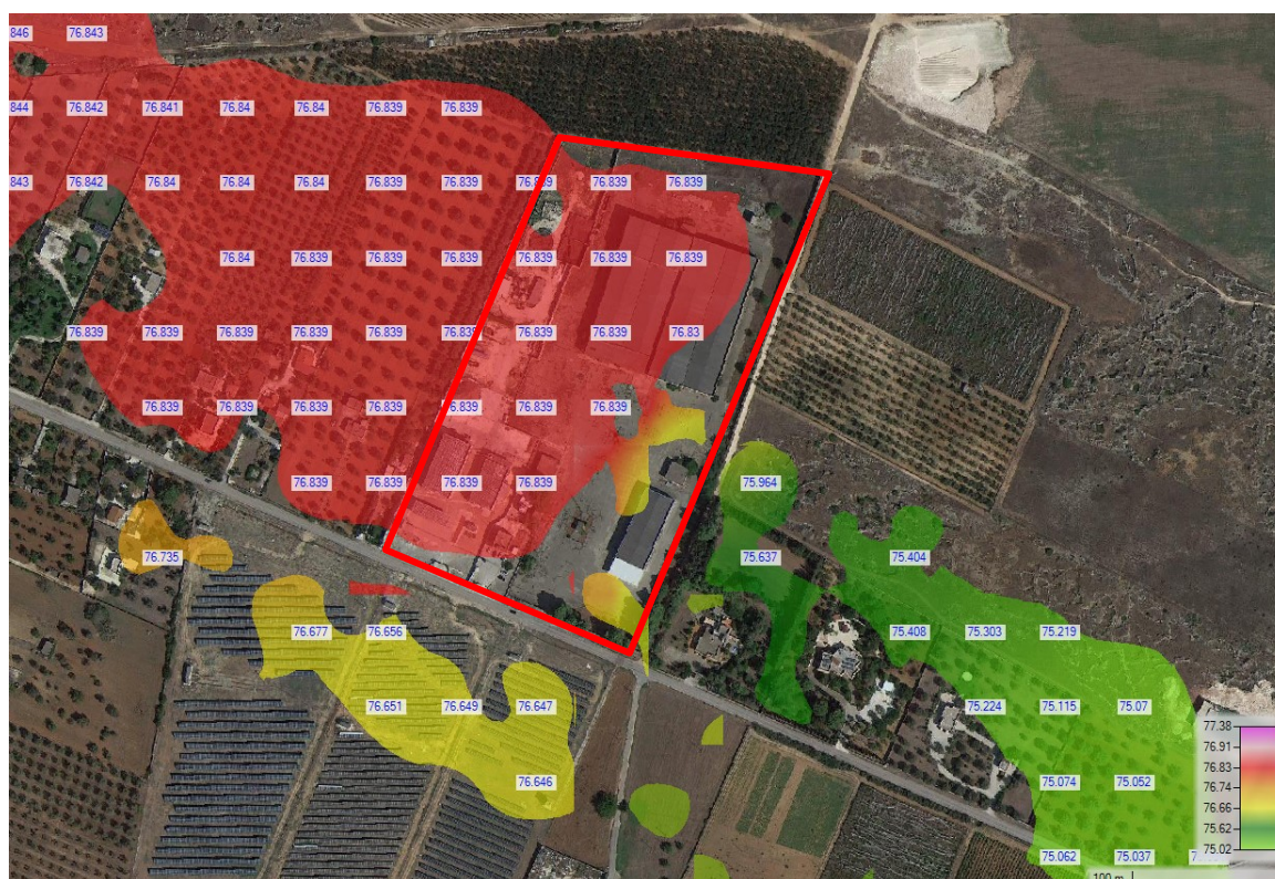
Pianta della W.S.E. in m s.l.m. (HEC RAS – Results Water Surface Elevation)
